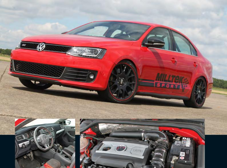
'The major boost, quite literally, to the power output of the EA888 2.0-litre TSI engine is from the use of a Garrett GTX2876 turbocharger to pump out more than double the 2.0 TSI engine's original power output...'
